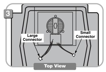
During the assembly you will be making two electrical connections. Identify the two connectors coming from the front panel.
